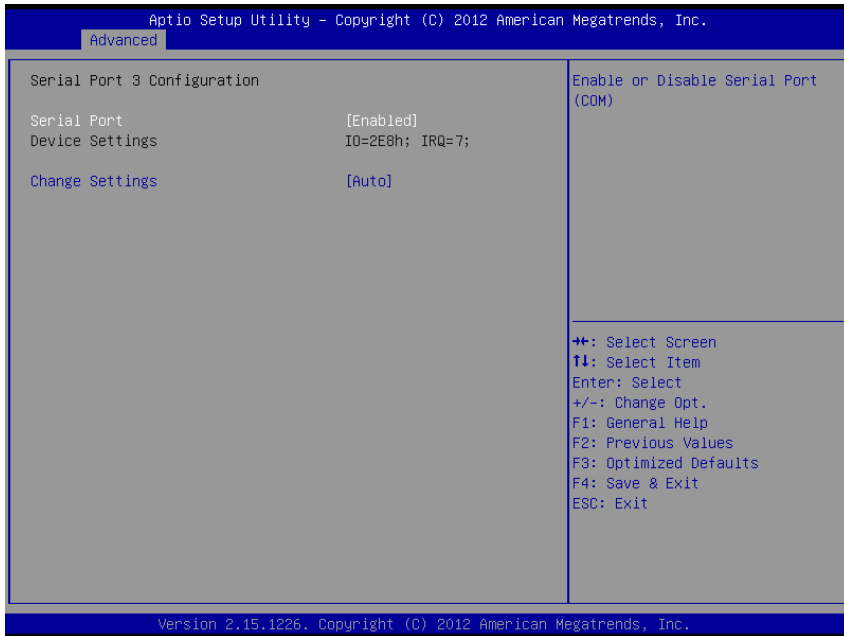
Serial Port 3 Configuration screen
