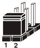
Jumper Block 1-2 pin close(enabled) Looks like this
