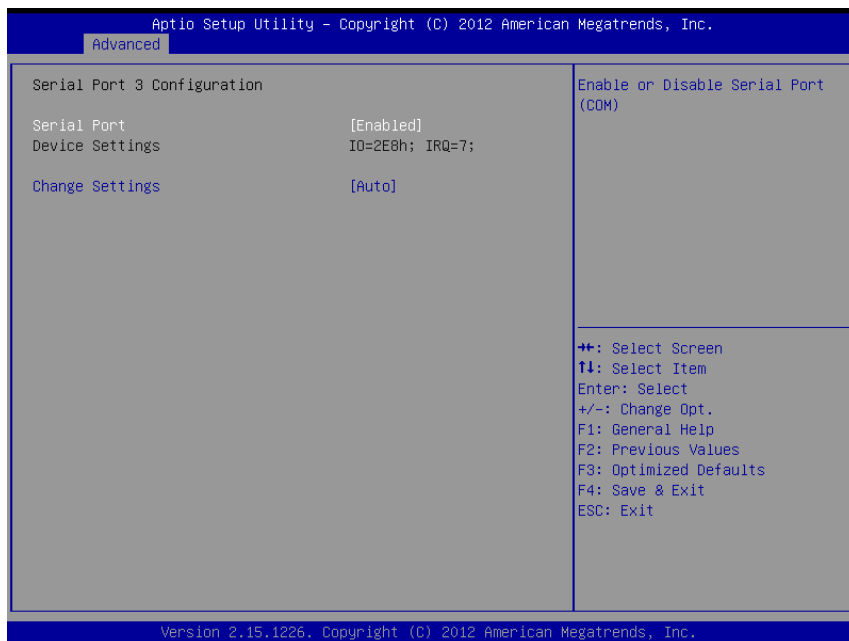
NCT6106 Super IO Configuration - Serial Port 3 Configuration Screen
