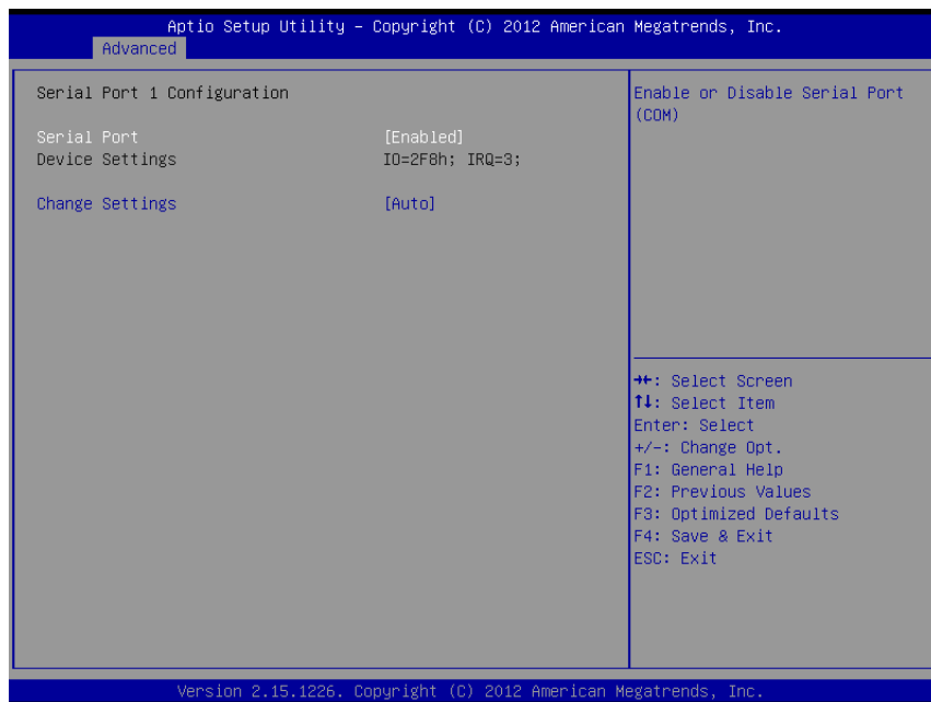
NCT6106 Super IO Configuration - Serial Port 1 Configuration Screen
