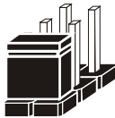
Jumper Block 1-2 pin close(enabled) Looks like this
