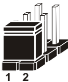
Jumper Block 1-2 pin close(enabled) Looks like this
