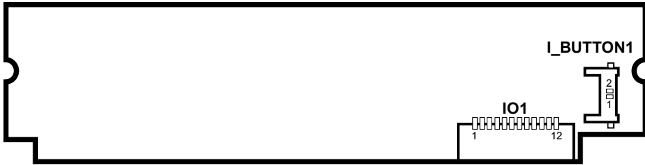
MB-3012 MSR Board Component Locations
