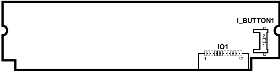
MB-3012 MSR Board Component Locations
