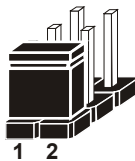
Jumper Block 1-2 pin close(enabled) Looks like this
