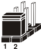
Jumper Block 1-2 pin close(enabled) Looks like this
