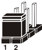
Jumper Block 1-2 pin close(enabled) Looks like this
