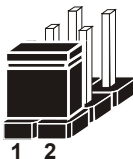
Jumper Block 1-2 pin close(enabled) Looks like this
